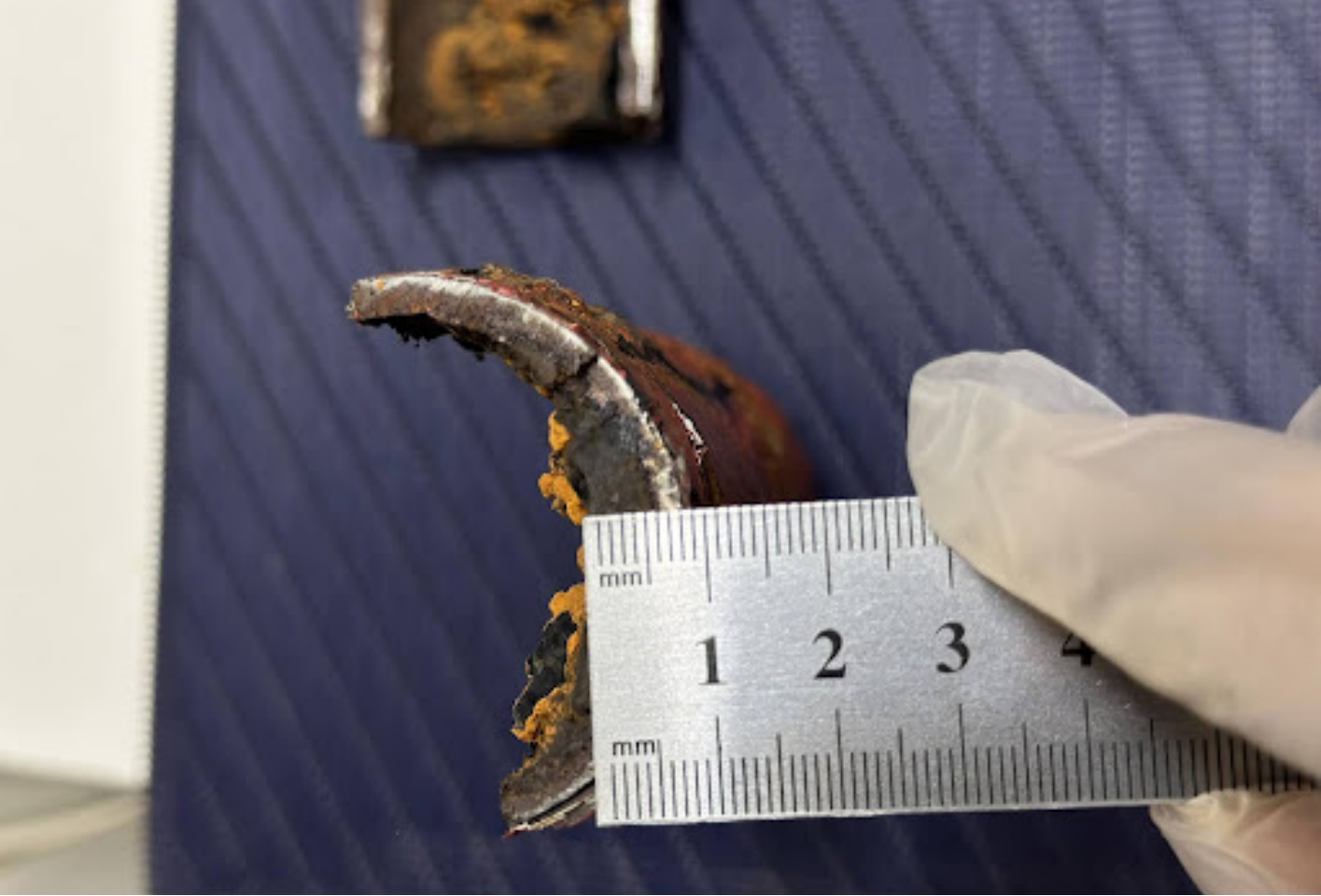
Figure -4 Longitudinal view of the carbon steel spool illustrating severe internal corrosion buildup. The accumulation of corrosion products has considerably restricted the internal diameter. Stratified corrosion layers consisting of porous FeOOH outer phases and darker magnetite-rich inner layers are present. Pitting cavities beneath tubercles indicate localized under-deposit corrosion.
